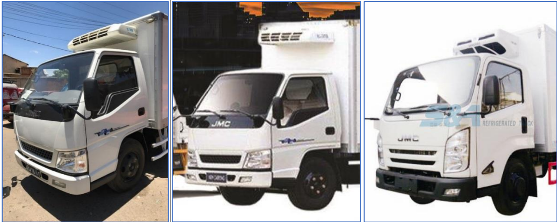
Vehicle purchased by MSANP (left) said to be 14m 3 . Same as that sold by the vendor, as per their catalogue (centre) with dimensions of 4,300 x 1,780 x 1,650, or 12.63m 3 . Contrast with actual 14m 3 vehicle not sold by the vendor (right).
